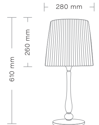
RETRO Lampa nocna/ Small table lamp max 1 x 40W Gwint/Chip: E27 Zasilanie/Power: 230V
